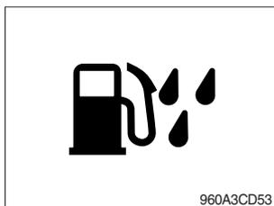
① This warning lamp lights ON when the water separator is full of water or malfunctioning.
