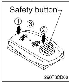
(1) This switch is used to select the regeneration function of the DPF.
